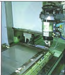
■a. X-Z軸の補間精度:20nm
