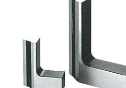
精密スクエアー (大小各1個) Rectangular block (Each 1 piece for Large/Small) 大(L): 87×72×20mm 小(S): 50×40×15mm
